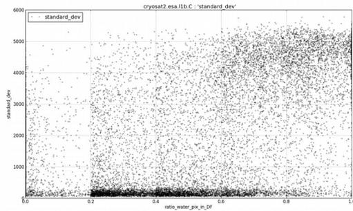
**Figure 6:** Standard Deviation of the Gaussian PDF fitting the RIP versus Water Fraction in CryoSat-2 Baseline-C L1B Beam-Doppler footprints over the Downstream Manaus section of the Amazon river. About 16000 records are displayed here to cover the 5 Water Fraction classes (3200 individuals per class).
