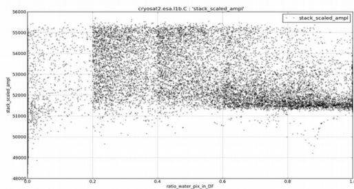
**Figure 5:** Scaled amplitude of the RIP versus Water Fraction in CryoSat-2 Baseline-C L1B Beam-Doppler footprints over the Downstream Manaus section of the Amazon river. About 16000 records are displayed here to cover the 5 Water Fraction classes (3200 individuals per class).
