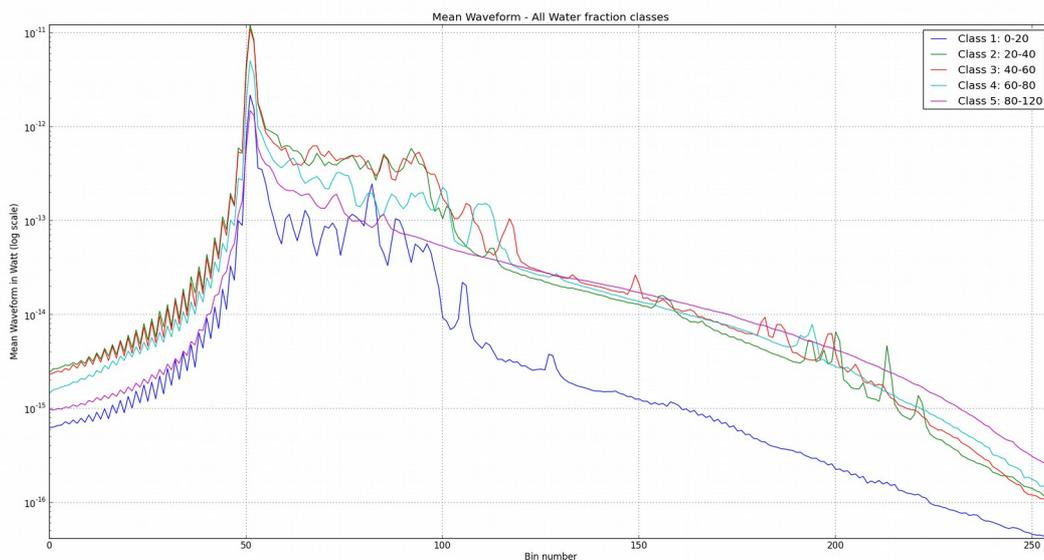
**Figure 3:** CryoSat-2 SAR Mode Baseline-C mean power waveforms in Watt for the 5 Water Fraction Classes. Ordinates axis in log10 scale.
