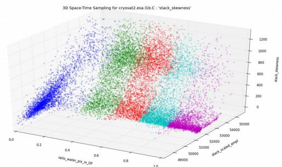
**Figure 9:** Skewness of the RIP versus Scaled Amplitude and the WFR in CryoSat-2 Baseline-C L1B Beam-Doppler footprints over the Downstream Manaus section of the Amazon river. About 16000 records are displayed here to cover the 5 Water Fraction classes (3200 individuals per class).
