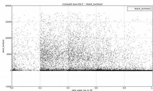
**Figure 7:** Kurtosis of the RIP versus Water Fraction in CryoSat-2 Baseline-C L1B Beam-Doppler footprints over the Downstream Manaus section of the Amazon river. About 16000 records are displayed here to cover the 5 Water Fraction classes (3200 individuals per class).
