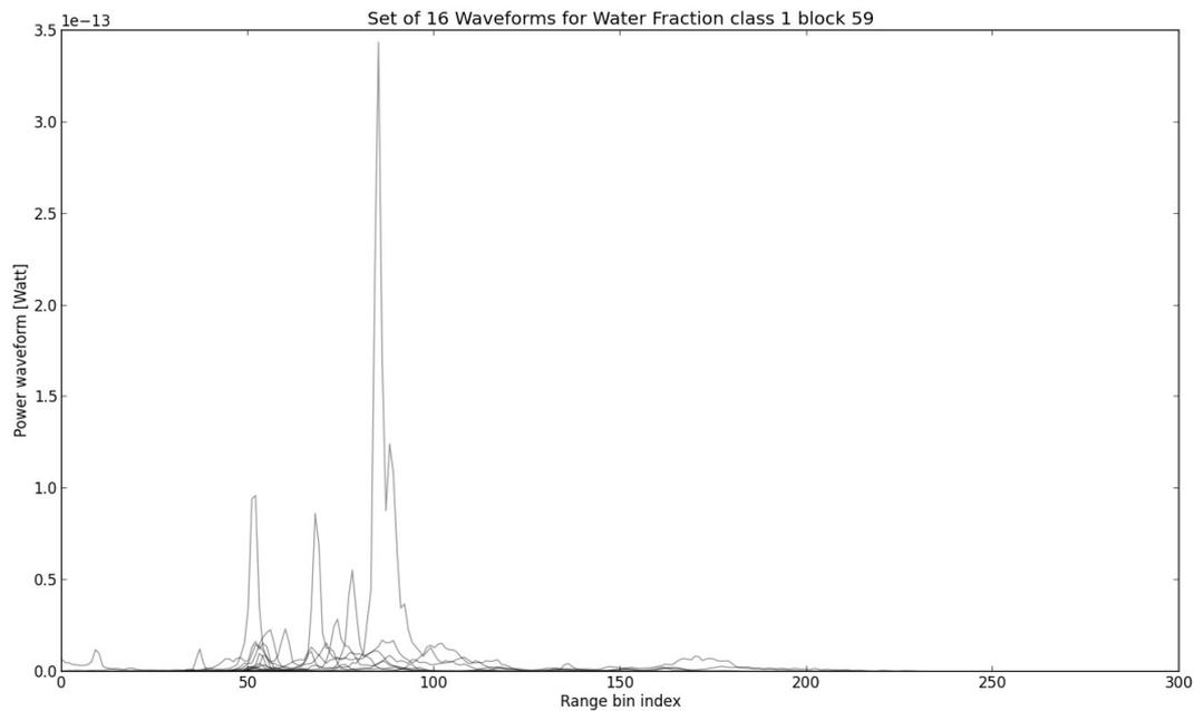
**Figure 4:** Set of CryoSat-2 Baseline-C L1B power waveforms in Watt for Water Fraction class 1 over Manaus downstream Amazon in 2014.
