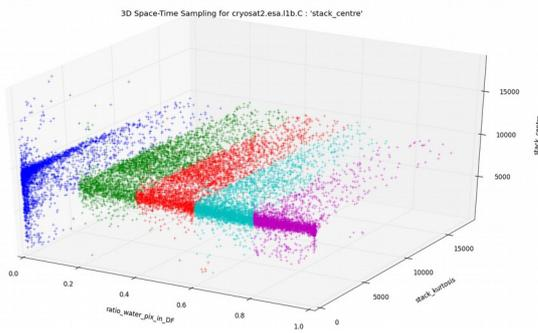
**Figure 10:** Centre of the RIP versus Kurtosis of the RIP and Water Fraction in CryoSat-2 Baseline-C L1B Beam-Doppler footprints over the Downstream Manaus section of the Amazon river. About 16000 records are displayed here to cover the 5 Water Fraction classes (3200 individuals per class).
