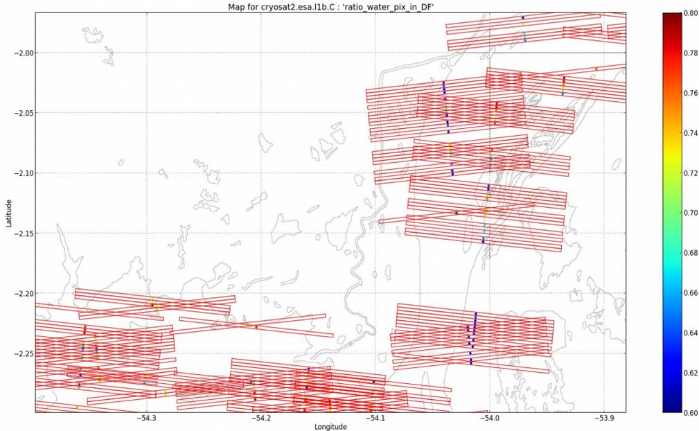
**Figure 1:** CryoSat-2 Baseline-C Beam-Doppler limited footprints (20Hz records) over downstream Amazon together with SWBD water masks and a central dot whose color indicates the water fraction (60-80%) in each footprint.
