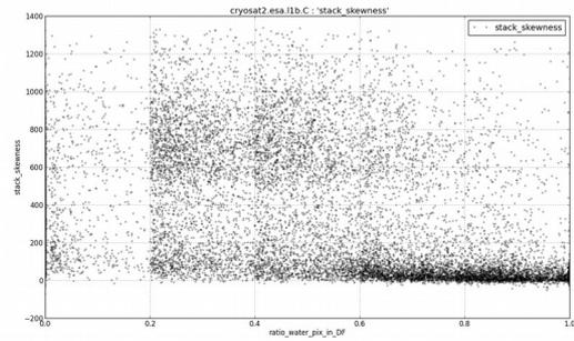
**Figure 8:** Skewness of the RIP versus the Water Fraction found in CryoSat-2 Baseline-C L1B Beam-Doppler footprints over the Downstream Manaus section of the Amazon river. About 16000 records are displayed here to cover the 5 Water Fraction classes (3200 individuals per class).
